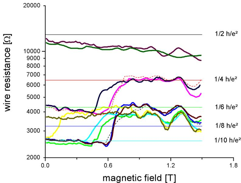
Fig. 3: Wire resistance versus magnetic field for a 400 nm wide, 2  $\mu\text{m}$  long wire structure. Different curves correspond to different illumination intensities of the nanostructure with a infrared light emitting diode.
