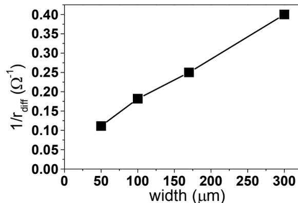
Fig. 3: Inverse differential resistance  $1/R_{diff}$  as a function of device width (after [4]).
