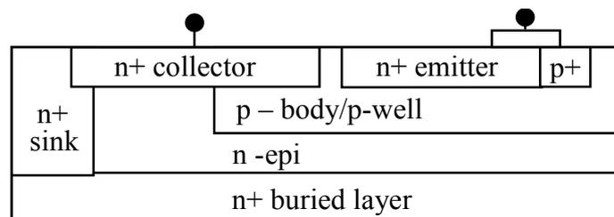
Fig. 1: Simplified cross sections of the studied device.
