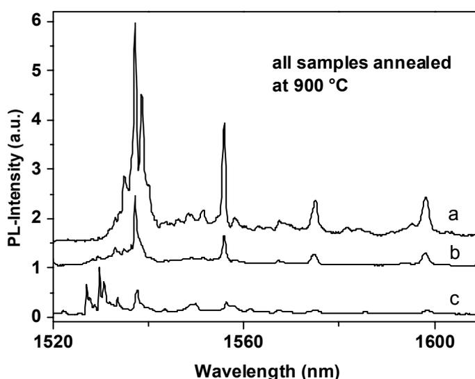
Fig. 2: (a) The cubic lines dominate the PL-spectra in the hydrogenated samples. (b) Spectra of a sample with low Er concentration and (c) of a reference sample (set 4) are shown. The lines at 1.53  $\mu\text{m}$  due to Er-O complexes are absent in the hydrogenated sample. Spectra shifted for clarity.
