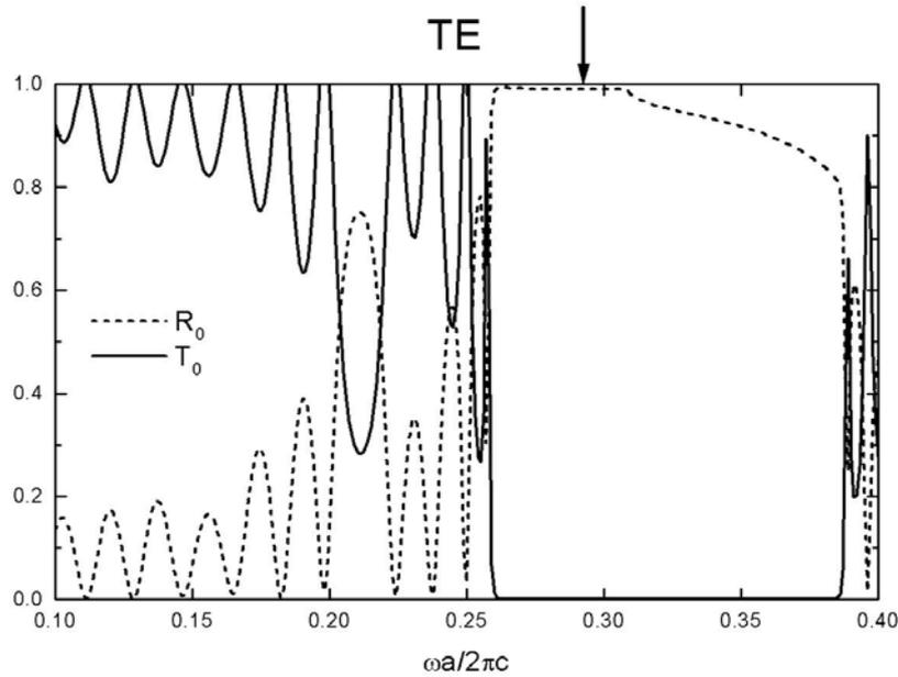
Fig. 1: Reflection at and transmission through a photonic crystal for TE (above) and TM polarization (below) as a function of normalized frequency
