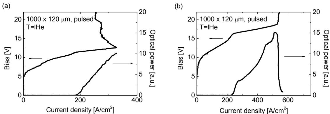
Fig. 1: IV-LI Characteristics. Comparison of the original (a) and the improved (b) structure
