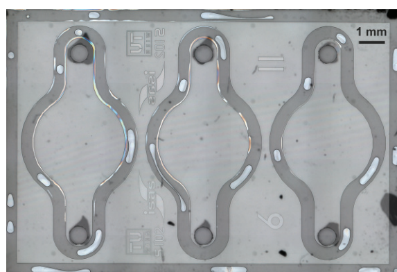
Fig. 3: Photograph of the 11x15x2 mm 3 microfluidic sample chip. Each chip consists of three sample chambers of 3.5 mm diameter and a volume of about 0.3 µL.
