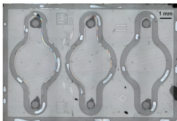
Fig. 3: Photograph of the 11x15x2 mm 3 microfluidic sample chip. Each chip consists of three sample chambers of 3.5 mm diameter and a volume of about 0.3 \mu L.
