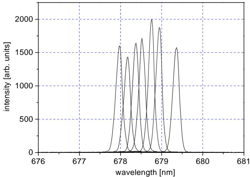
Fig. 3: The emission wavelength of the laser structures was adjusted (decreased) in steps of  $\approx 0.2$  nm in an interval of  $\approx 679.5$  nm to 678 nm by reducing the thickness of the waveguide on top of the laser diode.
