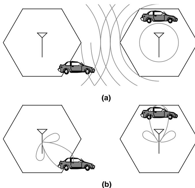
Fig. 3: (a) Omnidirectional antenna; (b) smart antenna.
