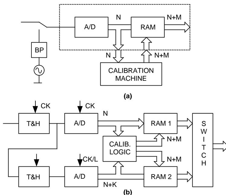
Fig. 8: (a) Off-line and (b) on-line digital calibration.
