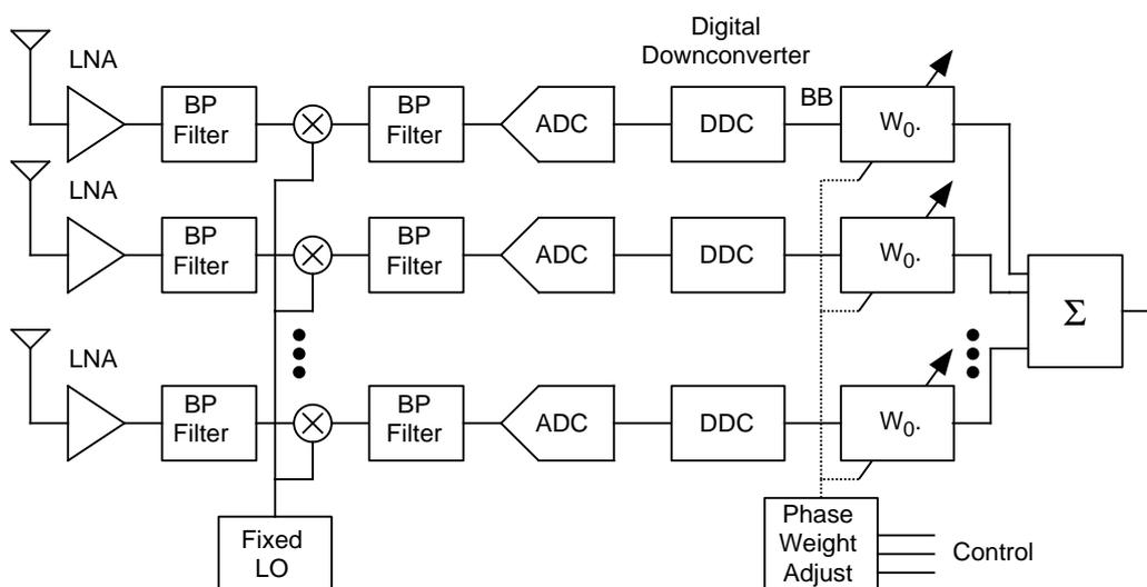
Fig. 4: Architecture of a digital smart antenna.
