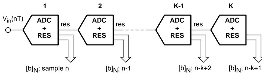
Fig. 7: Pipeline architecture.
