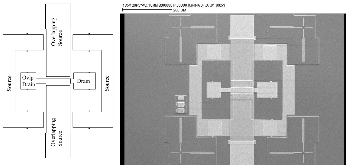
Fig. 2: Symmetric layout of the measurement circuit.
