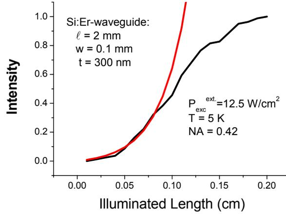
Fig. 3: Determination of the net gain of an optically pumped ( $\lambda = 514$  nm) Si:Er waveguide. In this sample, Er is incorporated as cubic interstitials making use of the hydrogen co-doping method. Black curve: experimental, red curve: model. As a result a net gain of  $35 \text{ cm}^{-1}$  is estimated.
