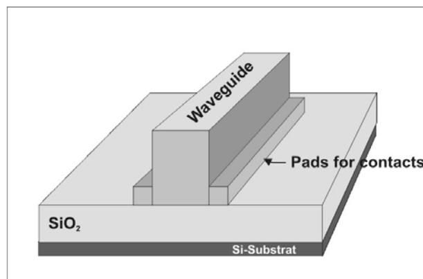
Fig. 1: Waveguide structure formed from SOI material; the dimensions are not to scale. The structure can be used for PL and EL measurements. For EL, electric contacts are put on top of the waveguide and on the pads on either side.
