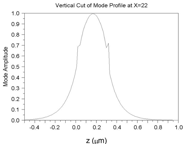
Fig. 2: Simulation of mode propagation in TE polarization in the waveguide structure shown in Fig. 1. Here “z” designates the vertical direction of the waveguide (x-axis: propagation direction).
