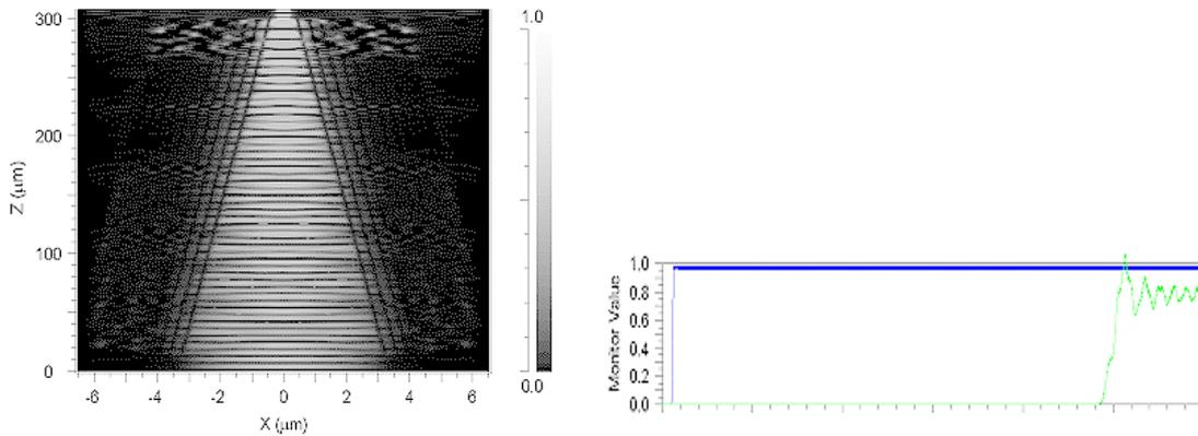
Fig. 2: Calculated efficiency of the coupler for TE modes.
