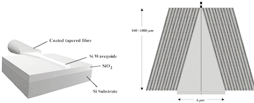
Fig. 1: Schematic drawing of the coupler
