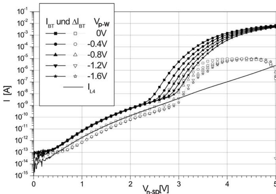
Fig. 2:  $I_{BT}$  for five different source-substrate bias-voltages. Empty symbols show the standard deviation of each measured value.
