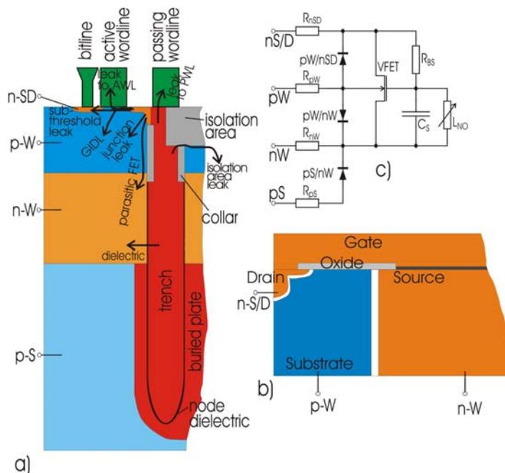
Fig. 1: n-SD...n-doped area of bypassed source and drain of the switching transistor; p-W...p-doped well; n-W...buried n-doped well; p-S...p-doped substrate
