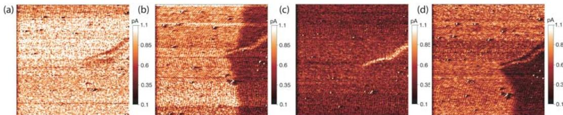
Fig. 2: Large area BEEM images showing magnetic domains in the vicinity of the switching field of the spin valve. Images (a) – (d) were recorded sequentially on the same position at different magnetic field levels of a minor loop. A film imperfection is visible on the upper right hand side of all images. The scan size is  $4 \mu\text{m} \times 4 \mu\text{m}$  and the images were recorded  $V_t = 1.8$  V,  $I_t = 20$  nA and  $T = 300$  K)
