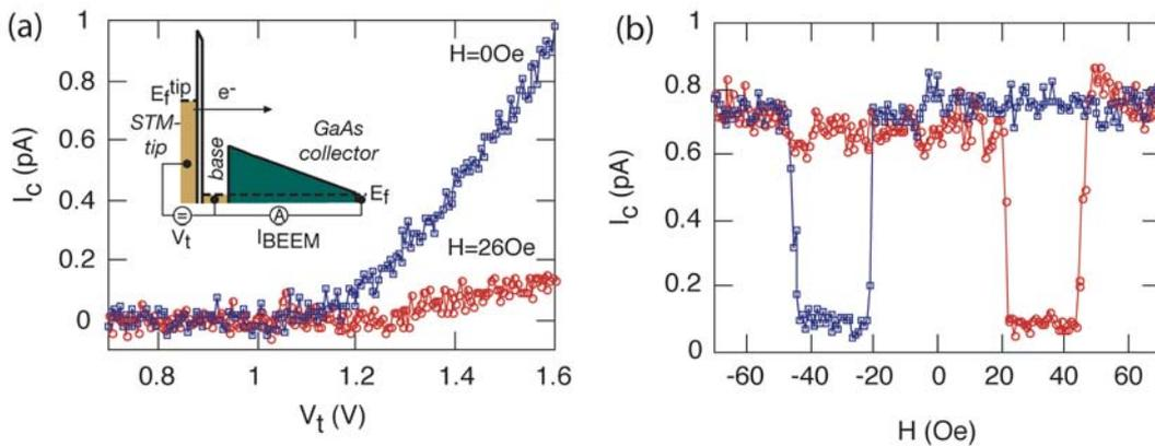
Fig 1: (a) Typical BEEM spectra recorded at  $H = 0$  Oe and  $H = 26$  Oe. The tunneling current  $I_t$  was 20 nA and the temperature 300 K. A schematic setup of the experiment is shown in the inset. (b) Collector current measured as a function of the magnetic field. ( $V_t = 1.5$  V,  $I_t = 20$  nA,  $T = 300$  K)
