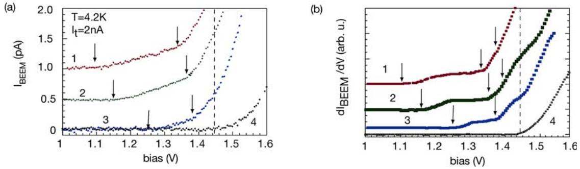
Fig. 3: (a) Measured BEEM spectra. Curves 1–3: RTDs with 40 Å, 30 Å, and 20 Å well width respectively. Curve 4: 100 Å thick AIAs single barrier. The arrows indicate the positions of the resonant levels; the dashed line marks the X-valley at the Au-GaAs interface. (b) First derivative of the spectra shown in (a).
