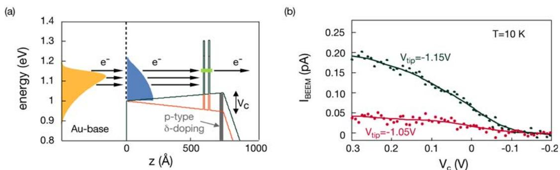
Fig. 1: (a) Band profile of the sample used for the electron refraction measurement, sketched for the unbiased sample and for a positive collector voltage, which lowers the band profile. Also indicated are the electron energy distribution in the Au base layer and the one in the GaAs, showing the massive broadening caused by the refraction. (b) Measured electron energy distribution in the GaAs for two different tunnel voltages.
