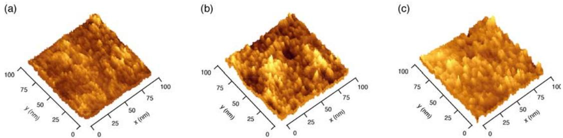
Fig. 4: BEEM images for AIAs single barriers with different doping concentrations. (a) undoped barrier, (b)  $N_D = 3e16 \text{ cm}^{-3}$ , (c)  $N_D = 1e17 \text{ cm}^{-3}$ .
