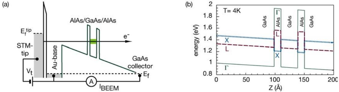
Fig. 2: (a) Sketch of the setup together with the  $\Gamma$ -band profile of a 30Å wide RTD sample, also indicating the position of the resonant level.
