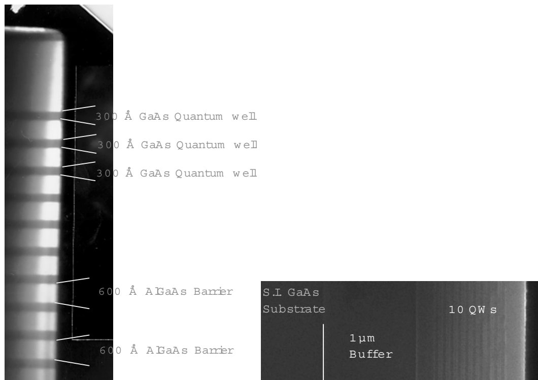
Fig. 4: TEM (left) and REM (right) pictures of MBE-grown Multiple Quantum Wells.
