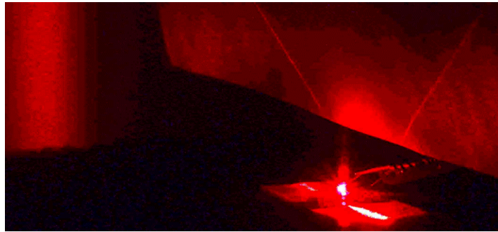
Fig. 2: The array elements emit via the surface. The intensity emitted per solid angle via the surface beam is five times larger than the one at the edges. Farfield pattern of a surface mode coupled laser: Two narrow surface beams and divergent spontaneous emission strike a paper screen (top) that is orientated parallel to the laser stripe contact. The divergent edge emission can be seen on the thermo electric cooling element and on a second paper screen (left-hand), which is orientated parallel to the cleaved facets.
