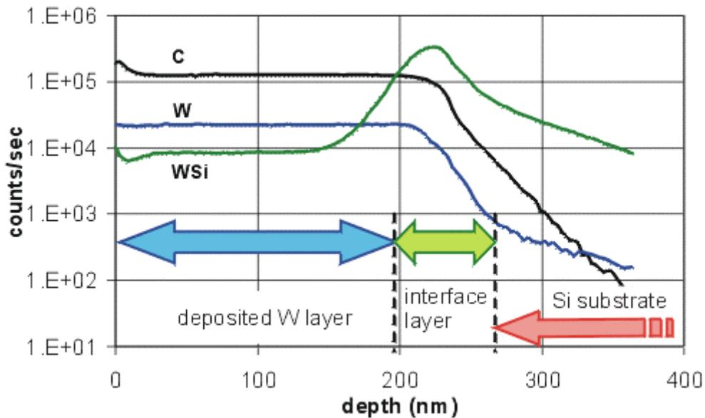
Fig. 3: SIMS depth profile of C, W and WSi. The pile-up in the WSi concentration indicates the atomic mixing at the interface layer.
