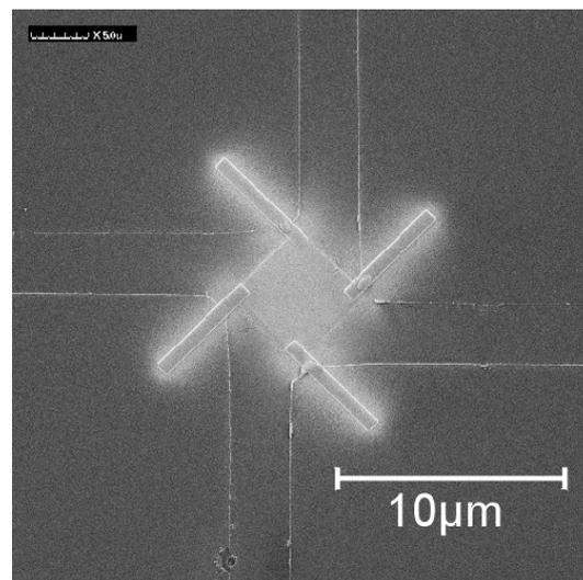
Fig. 4: SEM picture of a FIB tungsten test device.
