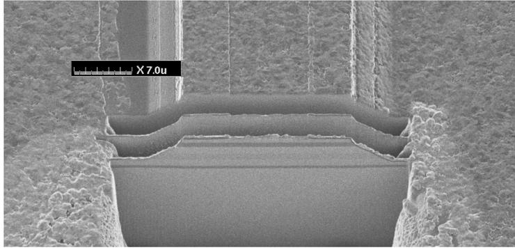
Fig. 2: FIB Image of the QCL with monolithic one dimensional photonic bandgap.
