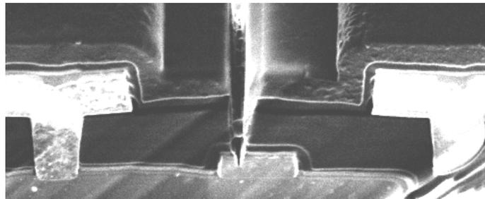
Fig. 1: Cross section of an inhomogeneous channel device.
