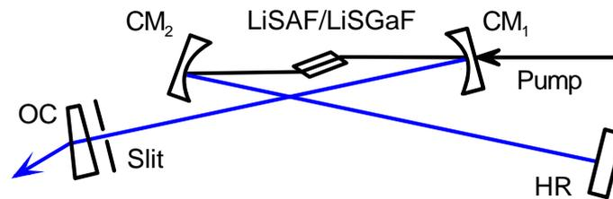
Fig. 1: Typical setup of a MDC femtosecond oscillator
