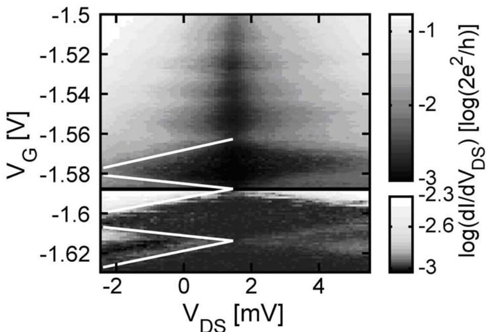
Fig. 4: Stability plot at 30 mK of the differential conductance through the dot as a function of the dc voltage  $V_{DS}$  between drain and source, and the gate voltage  $V_G$  applied to gates G1 and G2. Seven stability diamonds are clear visible.
