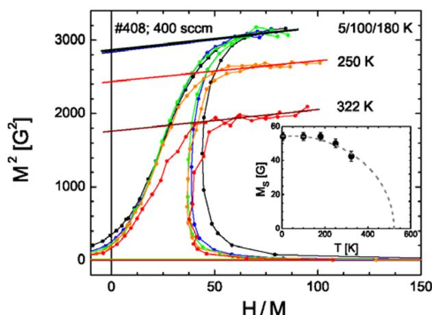
Fig. 3: Determination of the spontaneous magnetization at various temperatures obtained by plotting the square of the magnetization vs. the ratio of the magnetic field to the magnetization (Arrot plot). The inset shows the established spontaneous magnetization as a function of temperature. The extrapolation leads to an apparent Curie temperature of 500 K.
