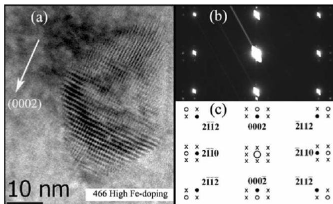
Fig. 1: (a) Elongated nanocrystal observed in an HRTEM image of Moiré fringes contrast. (b) SADP pattern acquired in the region around the precipitate along the (1010) zone axis; (c) the corresponding schematic graph for indexing of the diffraction spots.
