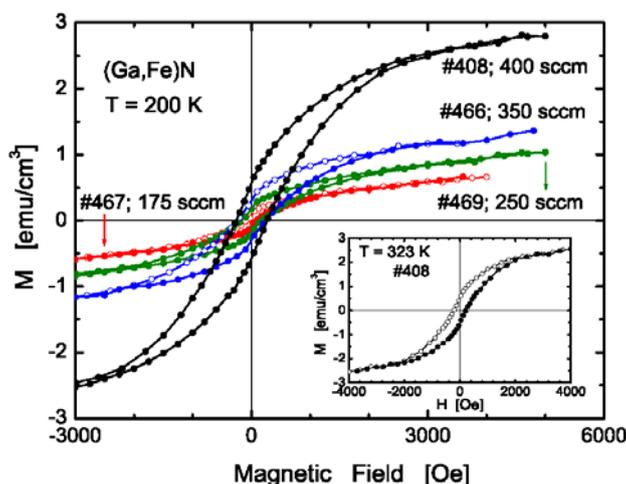
Fig. 2: Magnetization at 200 K for a series of (Ga,Fe)N samples with various Fe content (solid symbols). Inset: above room temperature  $M(H)$  for a sample with 3% Fe content.
