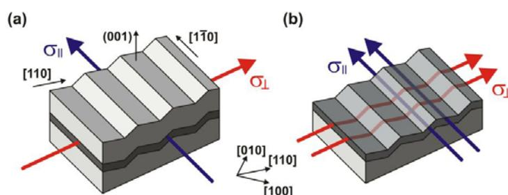
Fig. 1: Schematic drawings of a conventional p-SiGe modulation-doped structure with front-side doping. The conduction takes place at the upper interface of the SiGe-channel. The modulation of the channel yields expected differences in conductivity for measurements parallel ( $\sigma_{\parallel}$ ) and perpendicular ( $\sigma_{\perp}$ ) to the ripple structure.
