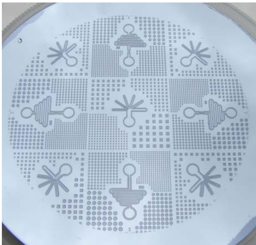
Fig. 1: Bonded 100 \mu\text{m} thick microfluidic structures on a 4 inch wafer without defects and deformation of channels.
