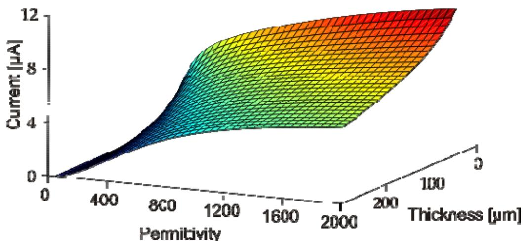
Fig. 2: FEM results of the electric current flowing into the detector for different values of ceramics permittivity and thickness. Simulation parameters for the channel were  $\epsilon_r = 80$  and electrical conductivity  $\sigma = 0.1$  S/m. This corresponds to an ion concentration of about 10 mM for the mentioned channel dimensions.
