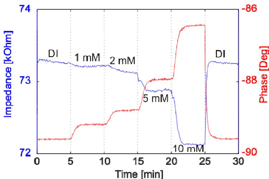
Fig. 3: Measured changes of impedance and phase over time for varying concentrations of an NaCl solution.
