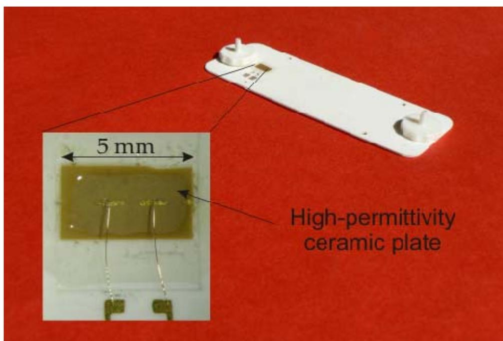
Fig. 1: LTCC device with planar detector-ceramic mounted in the recess above the channel (see inset). Electrode dimensions are 1 mm x 100  $\mu\text{m}$ . Electrodes were wire-bonded to contact pads positioned on the LTCC substrate.
