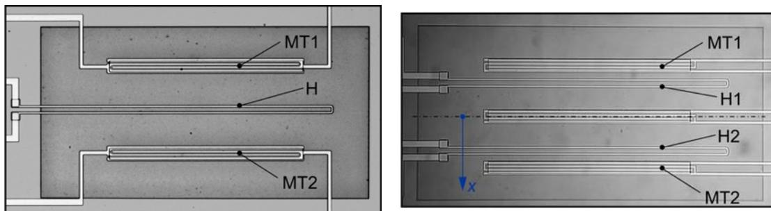
Fig. 2: Top view of the membrane area of a flow sensor featuring a common layout (left) and alternative design (right). The latter uses two equal-valued heating resistors together with the top and bottom thermistors. Highest sensitivity is achieved for flows in  $\pm x$ -direction.
