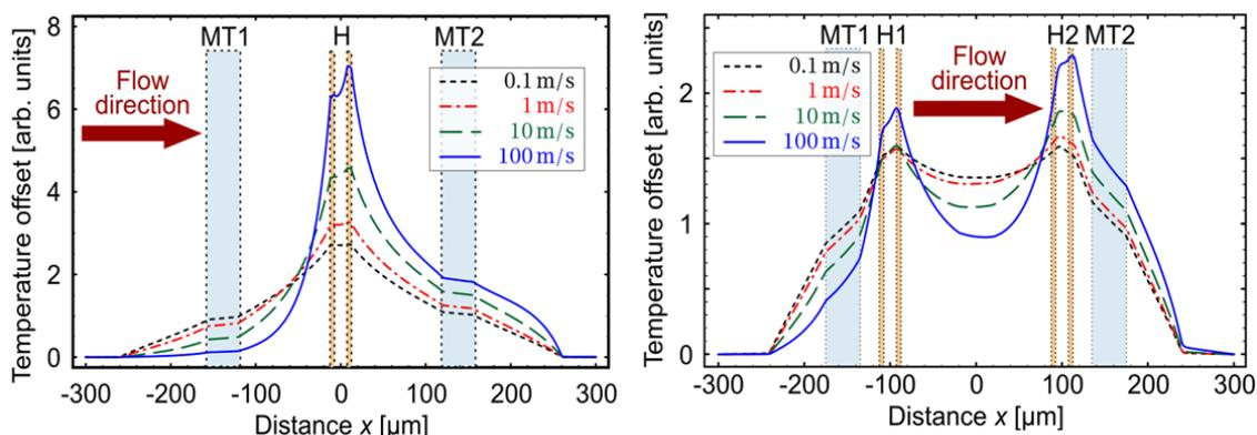
Fig. 3: Temperature profiles across the membrane region of flow sensors (left: standard design, right: alternative design) when operating in the enhanced CT mode.
