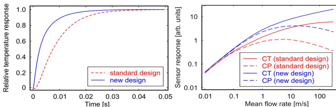
Fig. 4: Left: Zero-flow temperature sensor response to step like changes of the power dissipated by the neighboring heater. Right: Flow responses calculated for each sensor design and two operating modes
