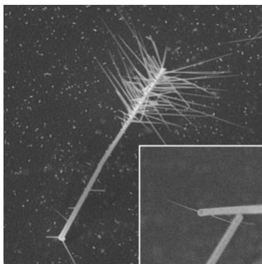
Fig. 4: GaAs nanowhiskers grown on a freestanding Si-NW trunk; MBE growth at 723 K for 524 s. The inset shows two GaAs whisker grown on opposite facets of a Si-NW; MBE growth at 723 K for 262 s.
