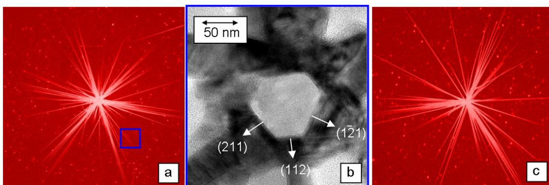
Fig. 2: (a) Top view SEM image of GaAs branches grown perpendicular to the free-standing Si-NW showing a 6-fold symmetry. (b) TEM image showing the cross-sectional hexagon of the Si-NW trunk with alternating wider and narrower vertical  $\{112\}$  facets normal to the  $[111]$  growth direction. (c) GaAs nanowhisker which grew preferably on the long facets of the Si-NW trunk with a quasi 3-fold symmetry.
