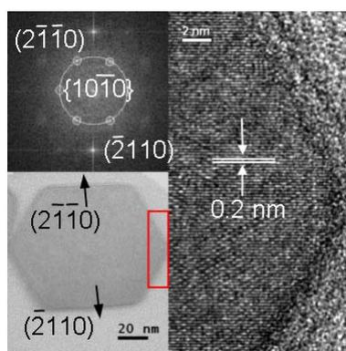
Fig. 3: Cross-sectional TEM and HRTEM image of a GaAs whisker and the respective diffraction pattern recorded along the nanowhisker axis.
