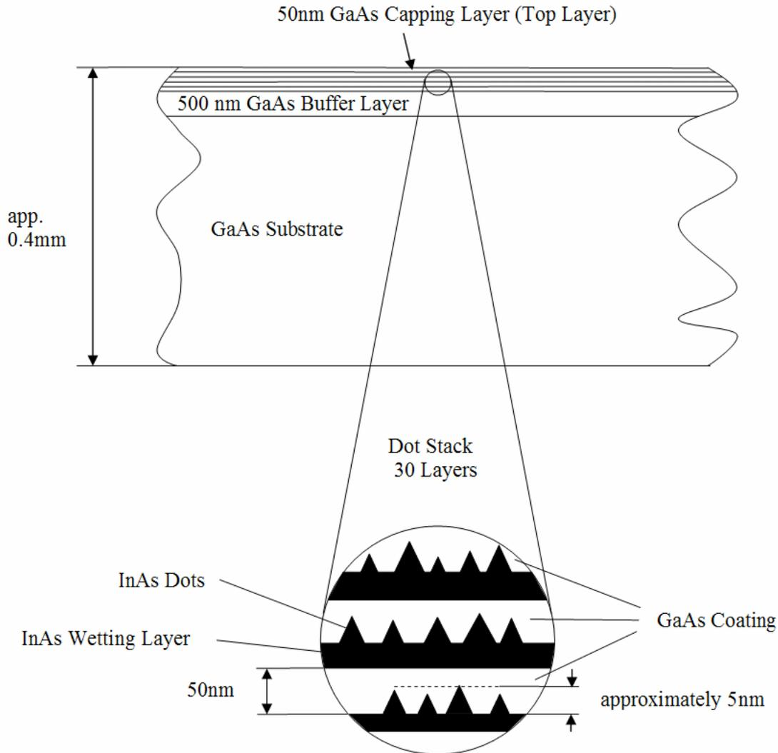
Fig. 1: Sample of self-assembled InAs / GaAs quantum dots
