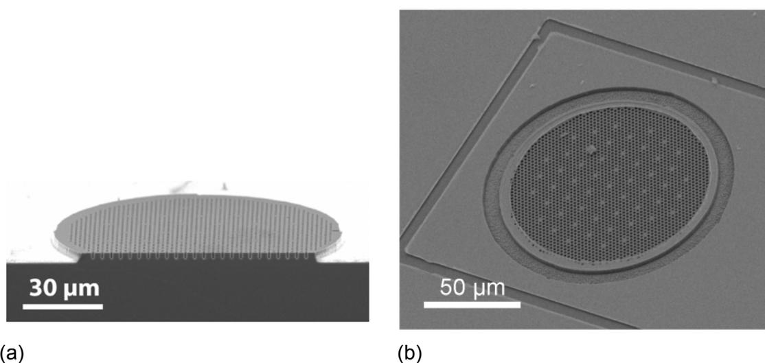
Fig. 1: Scanning electron pictures taken after the deep etching process (a) and of a finished device (b).
