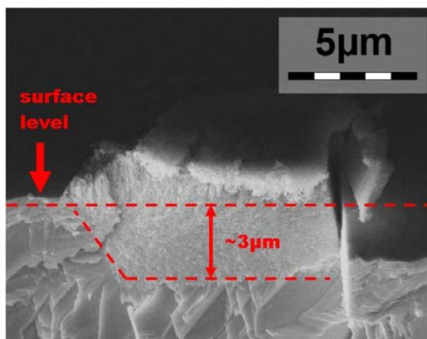
Fig. 2. SEM image of the cross sectional view of a FIB milled  $(10 \times 10) \mu\text{m}^2$  area accomplished by cleaving the sample. The porous network at the FIB exposed area using an ion fluence of  $3.1 \times 10^{18}$  ions/cm<sup>2</sup> reaches several micrometers in depth.
