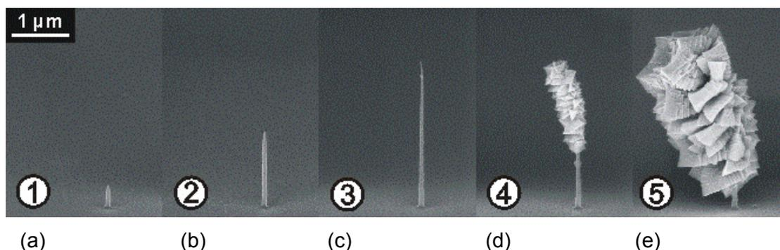
Fig. 1: Free-standing pillars deposited from  $\text{Fe}(\text{CO})_5$  with a 10 keV 1.97 nA focused electron beam. The  $\text{Fe}(\text{CO})_5$  in the supply line was 0.5 mbar resulting in a  $1.0 \times 10^{-5}$  mbar chamber pressure. The depositions are depicted by SEM at a 75° tilt after a deposition time of (a) 10 s, (b) 30 s, (c) 60 s, (d) 75 s and (e) 110s
