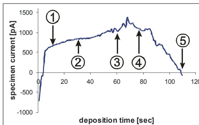
Fig. 2: Specimen current (current flowing off from the deposition area) monitored with progressing deposition time. The metal deposition was performed with a 10 keV 1.97 nA focused electron beam with a supply line pressure of 0.5 mbar  $\text{Fe}(\text{CO})_5$ . This current monitoring graph relates to Fig. 1.
