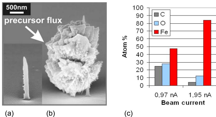
Fig. 3: Iron deposition at 10 kV with a 60  $\mu\text{m}$  aperture after 240 s (left) in low current mode 0.97 nA and (b) in high current mode 1.97 nA (image is 75° tilted) and chemical composition of these structures as determined by x-ray emission spectroscopy
