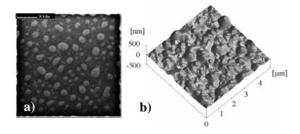
Fig. 1: (a) FIB-SEM image of a GaAs surface after FIB exposure of a 5 μm x 5 μm box with 50 keV Ga ions, (b) AFM topography of the GaAs sample after milling.
