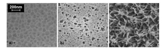
Fig. 3: GaSb surface evolution driven by ion fluence: depositing an ion fluence of 3x10<sup>13</sup> ions/cm² (a) leads to generation of hollow combs under a thin surface layer, increasing the fluence to 6x10<sup>13</sup> ions/cm² (b) results in a more and more porous layer and finally at an ion fluences of 3x10<sup>14</sup> ions/cm² a transformation into a sponge-like network built up of GaSb fibers with diameter in the range of 25 nm and Ga-rich precipitations takes place.
